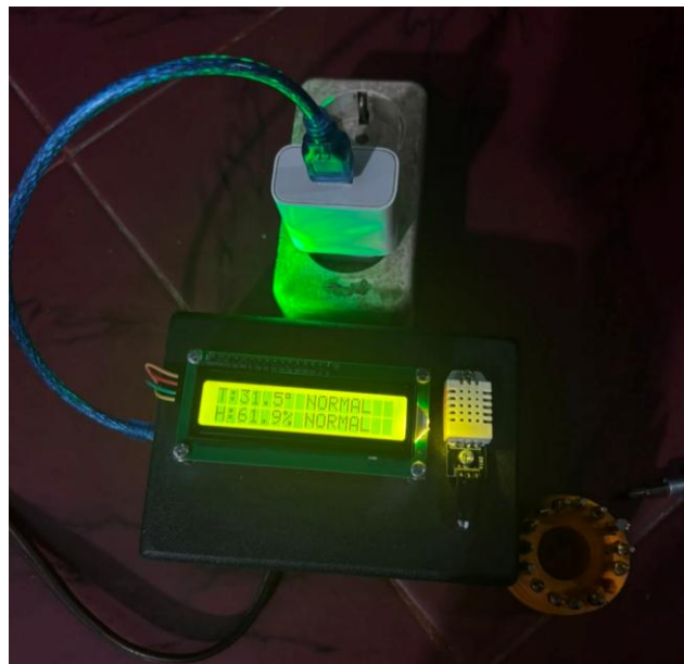
Fig. 7. Implementation of the proposed IoT-based temperature and humidity monitoring system.
