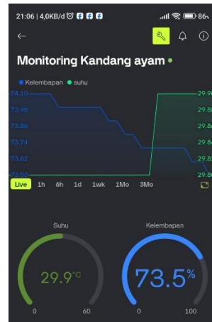
Fig. 8. Real-time monitoring interface using the Blynk platform.
