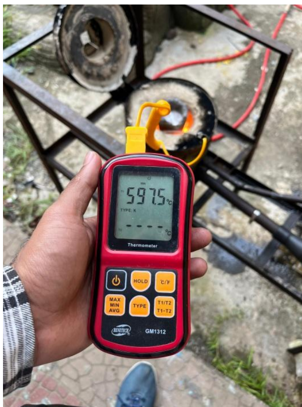
Fig. 4. Thermocouple Temperature Sensor Used in the Furnace System
