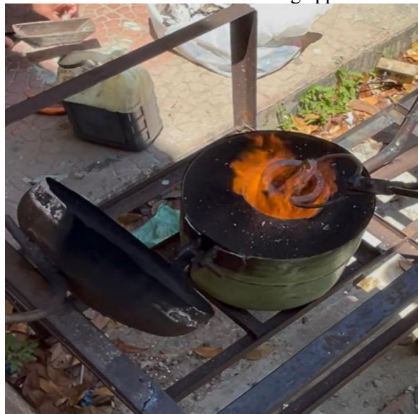
Fig. 2. Combustion Process of Metal Melting in the Furnace
