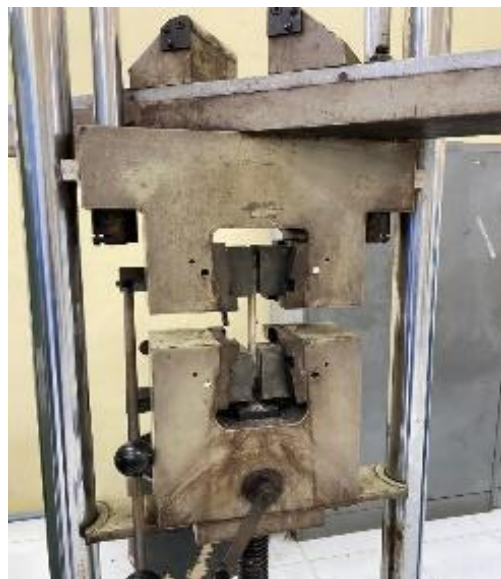
Fig. 1. Galdabini Tensile Testing Machine Used in This Study.
