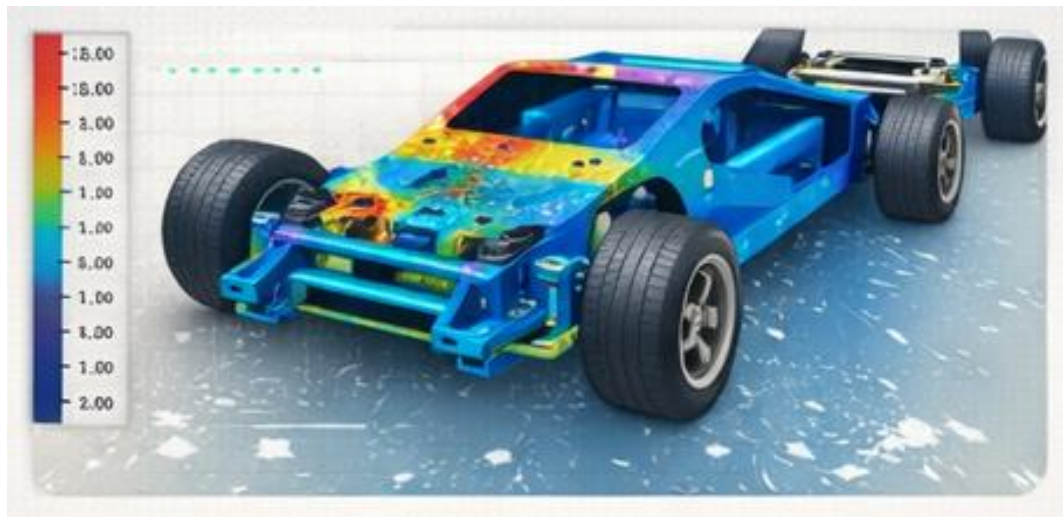
Figure 2. Von Mises stress on the EV chassis under dynamic load conditions
