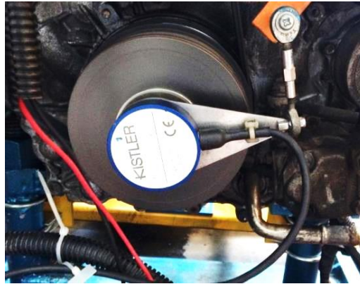
Figure 1: Kistler CAM crank angle encoder type 2613B1
