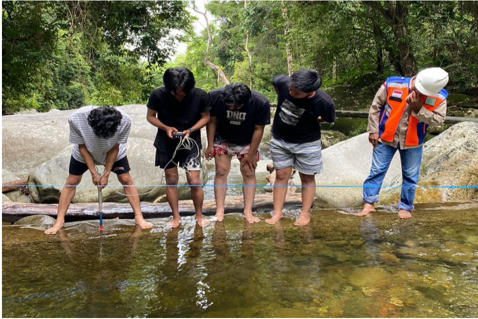
Figure 7: Field Measurement of Stream Flow for Micro-Hydro Power Site Assessment
